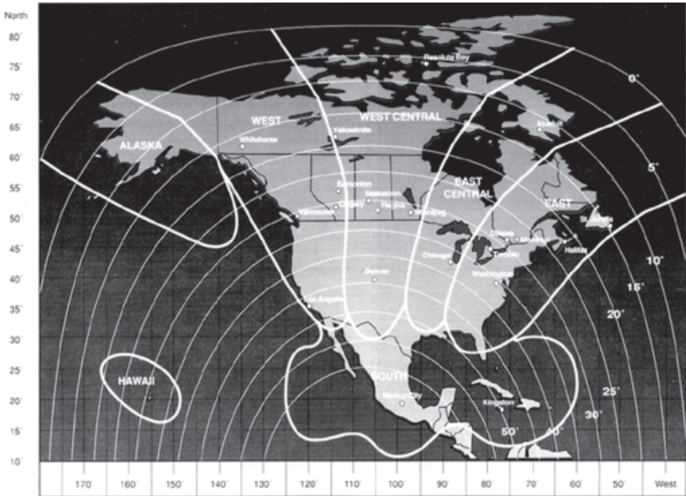
Map of the MSAT satellite's coverage pattern. Four east-to-west beams cover Canada and the United States. A south beam provides coverage throughout Mexico, the Carribean, and Central America. A dual-spot beam covers both Alaska and Hawaii.
